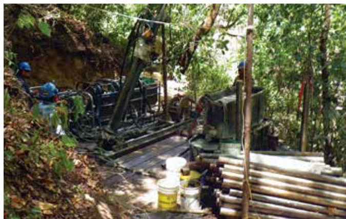
A small-footprint exploration drill site at San Sebastián
