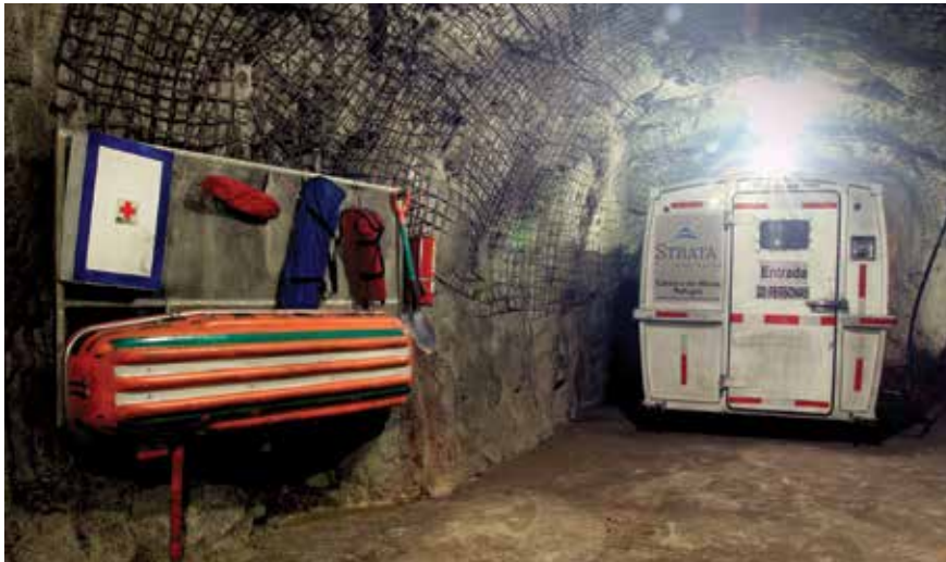
Mine rescue chamber underground at El Cubo
