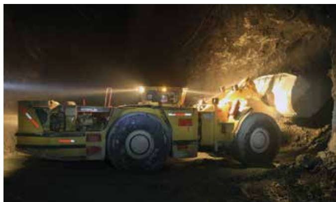
A scoop tram loading ore at Bolañitos
